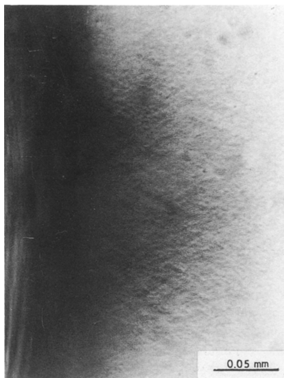
Figure 8 Optical micrograph of stress-whitened zone of 3.6 mm thick PVC with 15 p.p.h. experimental resin 5896 loaded at 28.2 MPa with the focus at the centre of the specimen.
